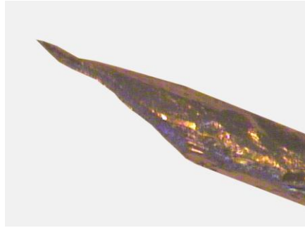
Fig. 6-23. Typical shape of a wire cutoff
