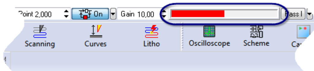
Fig. 7-6. Scanner extension indicator after approaching
