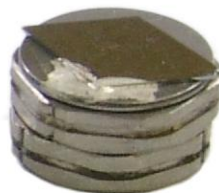
Fig. 6-3. Round substrate with the sample (fixation with conductive paste) on a stack of two magnetic sample holders
