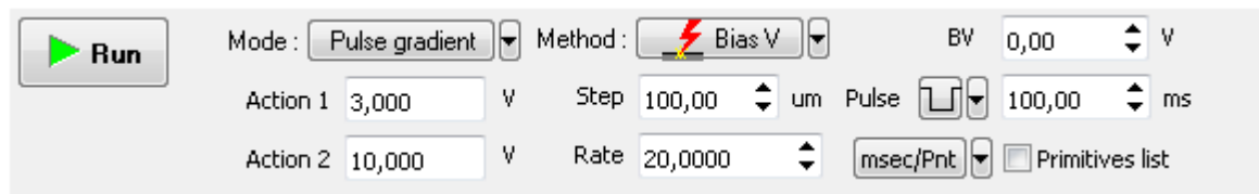
Fig. 12-42. Lithography Control panel. Select the pulse gradient charge lithography
