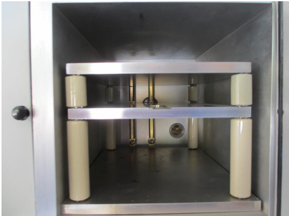
(above) Top Shelf is Grounded, Middle Shelf is Connected to the RF Power, and the Bottom Shelf is floating.
