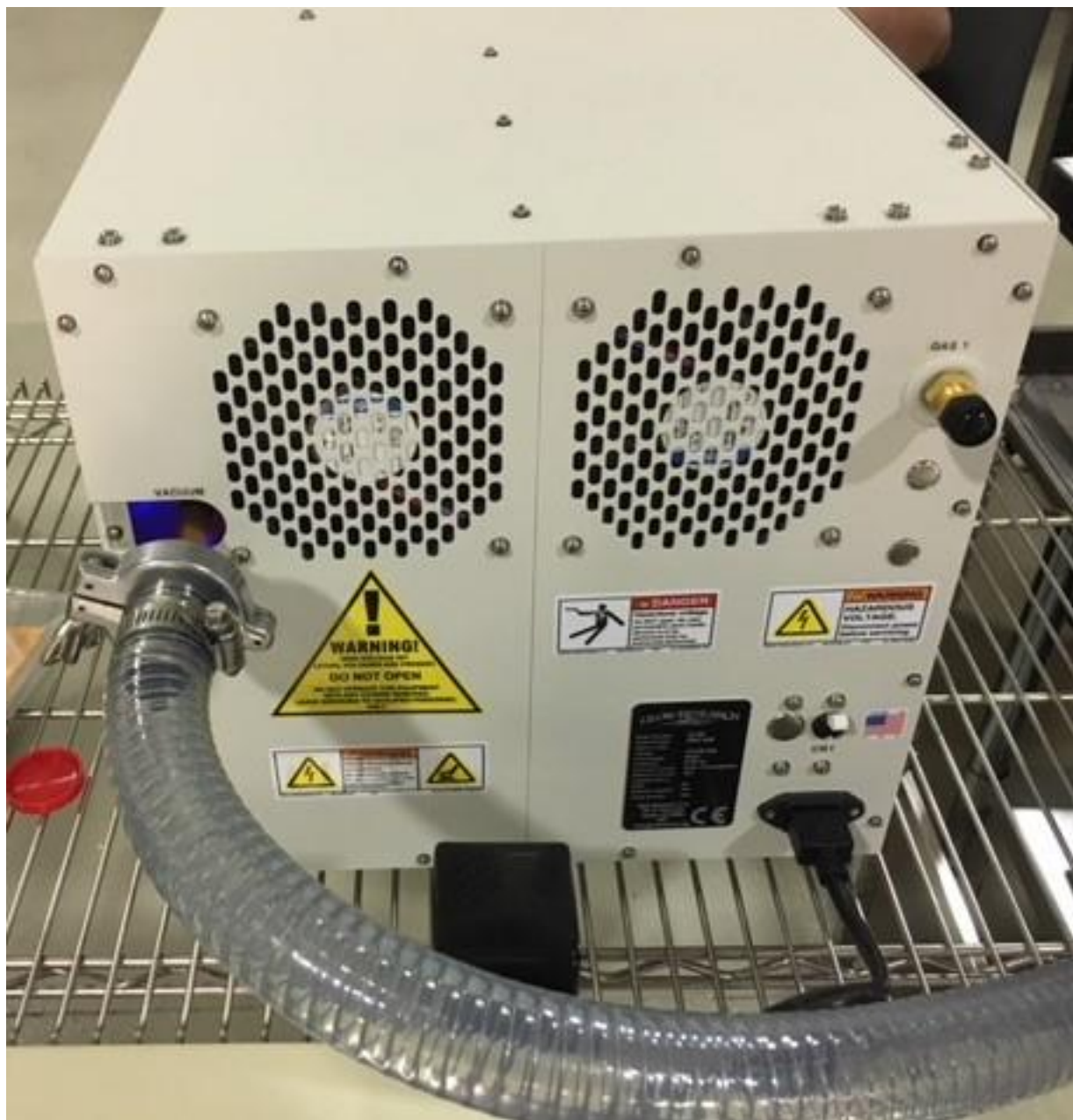
Back of Glow system showing KF-25 flange connection with vacuum hose
