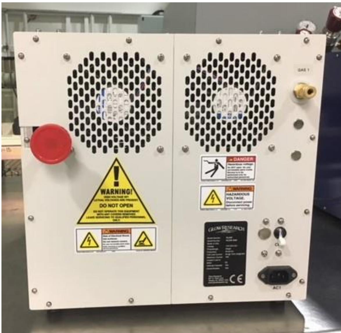
Back of GLOW system—KF-25 flange connection for vacuum, AC input, process gas input and breaker shown in the off position
