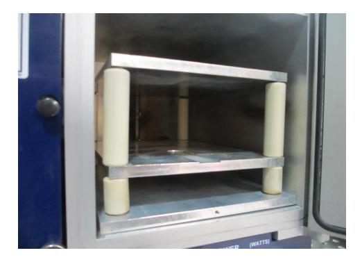
•The carrier above has a larger working space—the top electrode is ground and the lower middle shelf is powered for RIE type of processing
