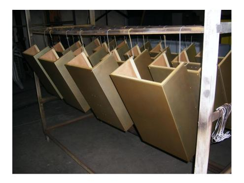
•Reliability starts with the conductive coating of the cabinet metal prior to the powder coat. This is critical for RF containment and RF reliability.
