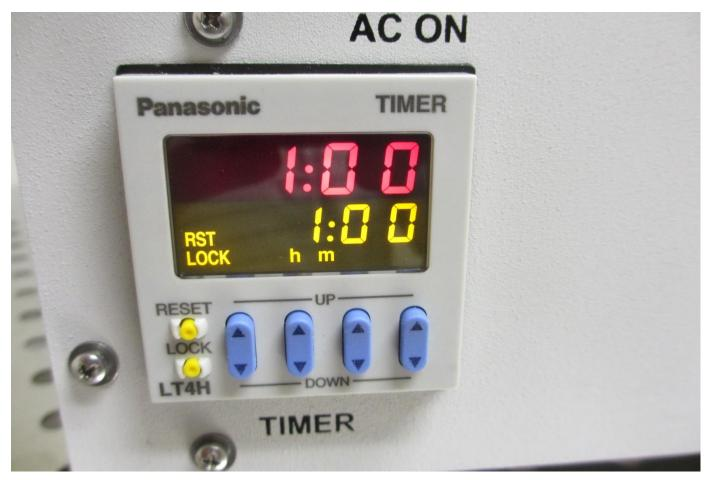
Process time can be set in minutes and seconds. RF processing will automatically stop at the set time limit.
