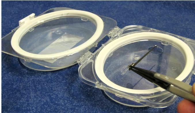
**Figure 3-22: Lifting the Stylus from Its Case**
