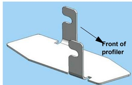
**Figure 3-17: Magnetic Shield Removed from Sensor Head**
