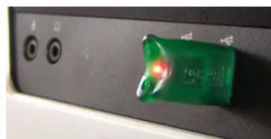
Figure 5-1: Software Key in a USB Port
