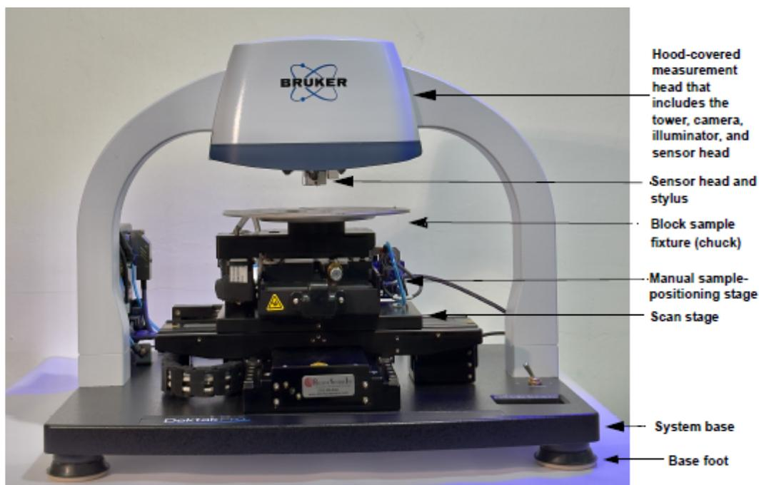
Figure 2-1: DektakPro Stylus Profiler with the Standard Manual X-Y Sample-Positioning Stage
