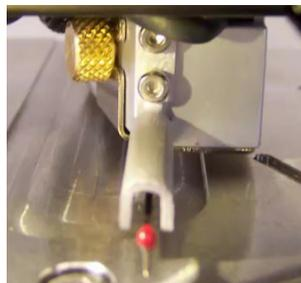
**Figure 3-14: Sensor Head and Stylus on the DektakPro Profiler**
