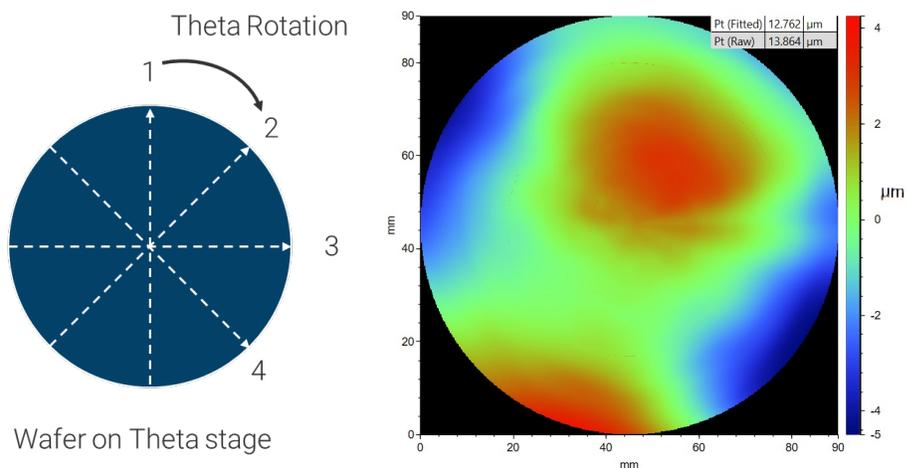
*On left, principle for Wafer Warpage Map. On right, resulting topography with high points in red and low points in blue.*
