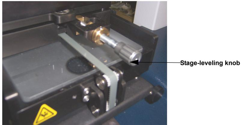
**Figure 3-9: Stage-Leveling Knob**
