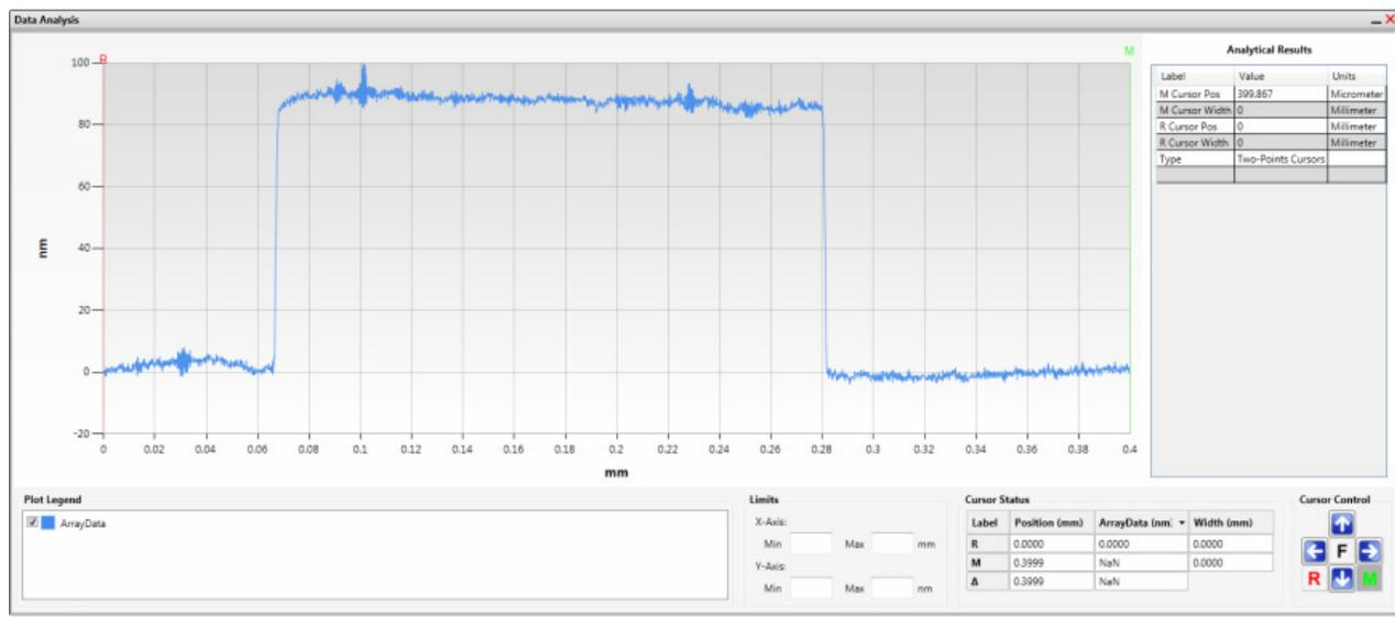
Figure 2-12: Output Display for a Single-Scan Measurement
