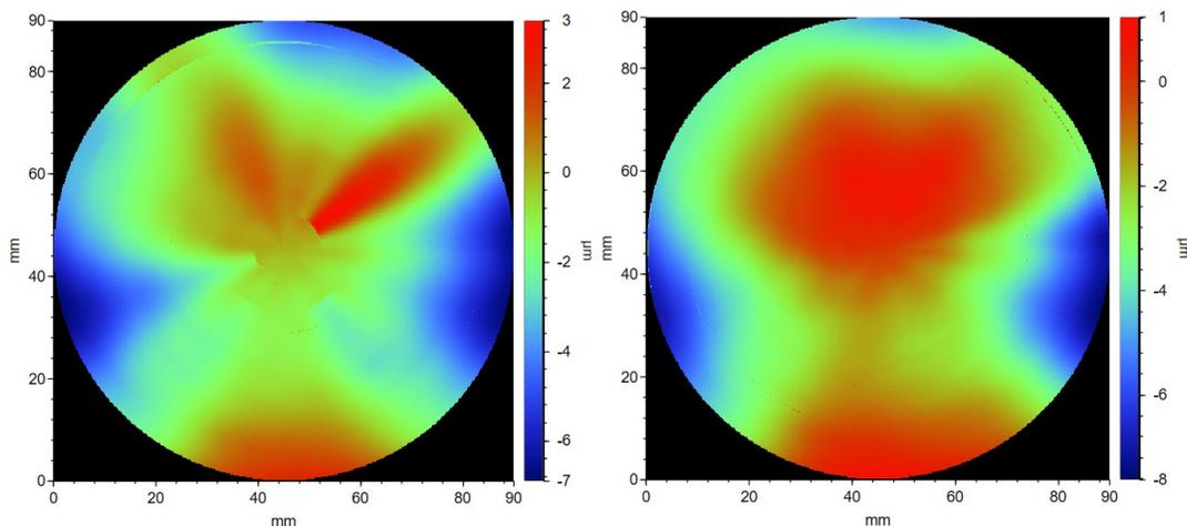
*Same sample without proper centering (Left) and with proper calibration (Right) of wafer center as well as center of theta rotation*
