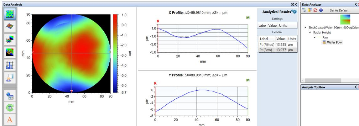
Since it is a real topography map, user can bring cursors to different locations as well as select radial section through right click on topography image. Each section can also show several useful parameters by showing the Watch List where local slope or radius of curvature between R and M cursors can be live worked out.
