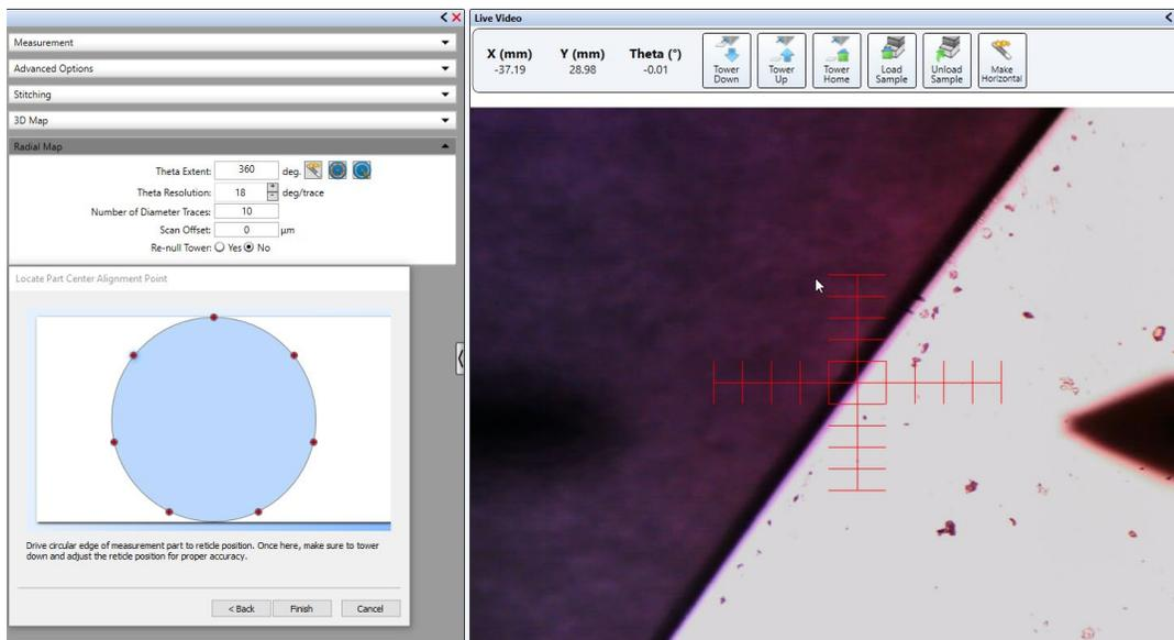
When all locations are done, click on Finish. Vision64 automatically drives stage such as stylus is located at defined center of sample. All the radial map measurement must start from this position. To recover this important position, conveniently click on button
